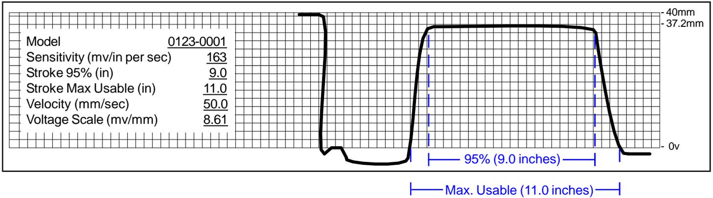
The Trans-Tek Series 100 Linear Velocity Transducers produce a DC output voltage proportional to the velocity of the magnet relative to the coil. These units are designed and tested to assure that they conform to prescribed specifications. Each unit is calibrated by our QC Dept., and a strip chart recording of the results is packaged with each unit.
